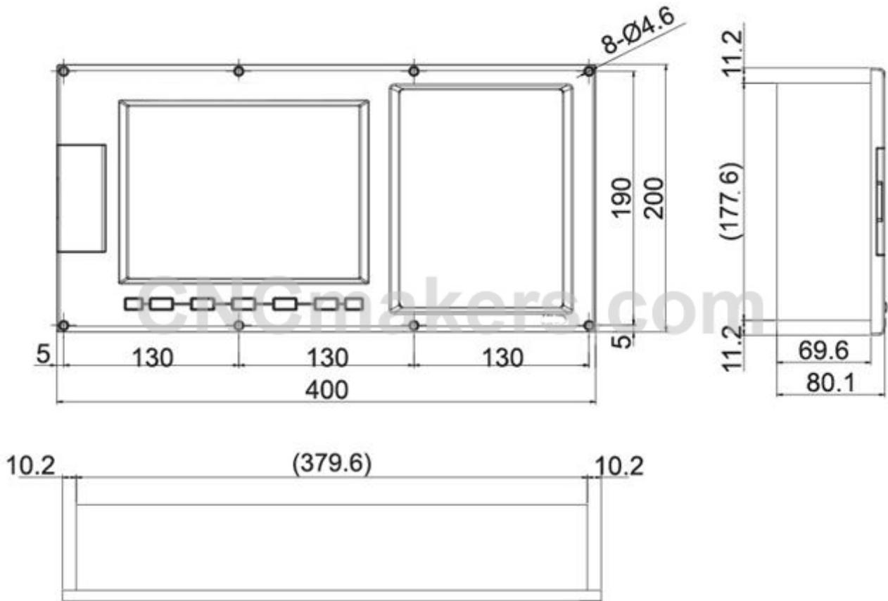
Machine control panel (pushed button) and additional panel :
