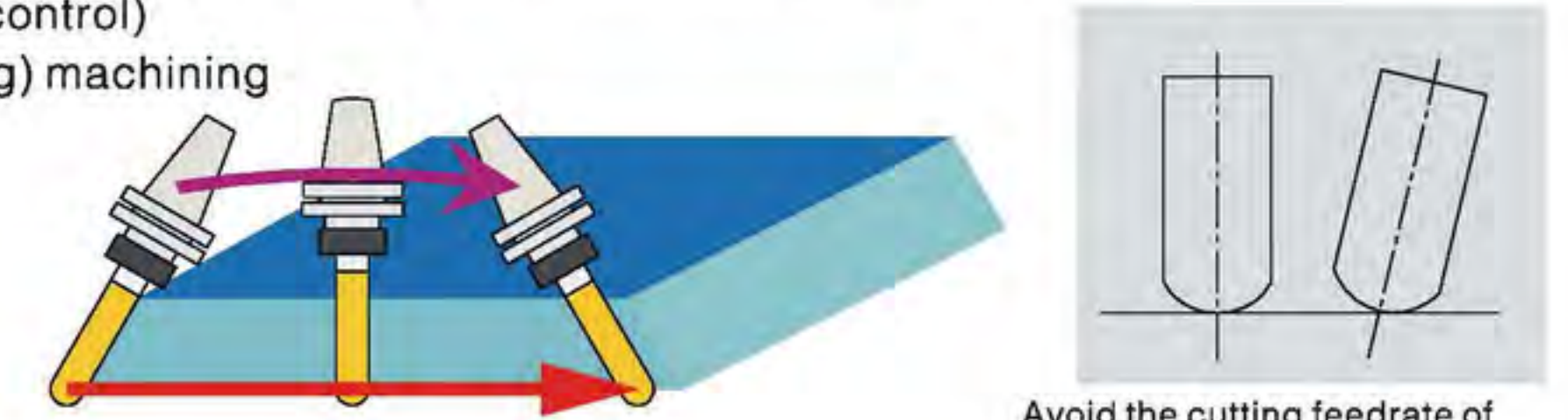
Higher efficiency when machining with tool side edge
